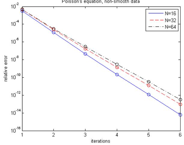
Figure 2: Relative error in solutions to Poisson's equation (19), (22), (23) computed by 2-node block KSS methods with residual correction.
