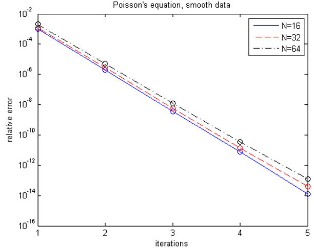
Figure 1: Relative error in solutions to Poisson's equation (19), (20), (21) computed by 2-node block KSS methods with residual correction.
