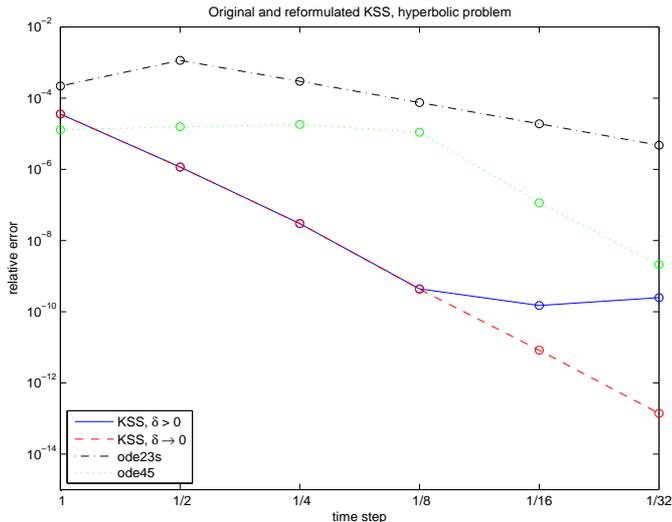
Figure 1: Estimates of relative error in the approximate solution of problem (20), (21) at  $t = 1$ , computed with the original KSS method from [11] with  $\delta_\omega = 10^{-5}$  (solid curve), the reformulated KSS method (dashed curve), the MATLAB solver `ode23s` (dotted-dashed curve), and `ode45` (dotted curve). In both KSS methods, 2-node Gaussian quadrature rules are used, and  $N = 64$  grid points are used for all methods.
