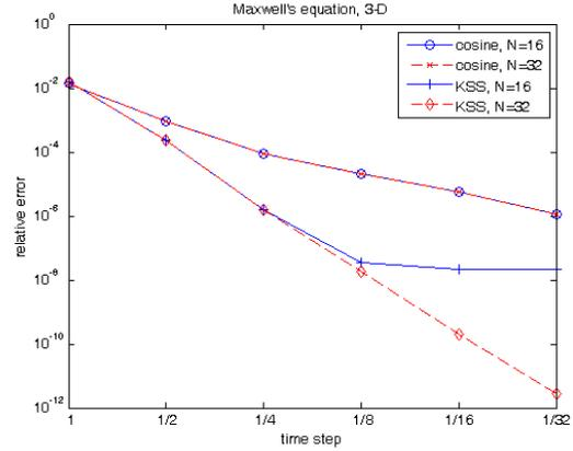
Figure 2: Estimates of relative error at  $t = 1$  in solutions of (19), (23) computed using a cosine method based on a Gautschi-type exponential integrator [13, 15] with 2 Lanczos iterations, and a 2-node block KSS method. Both methods compute solutions on an  $N^3$ -point grid, with time step  $\Delta t$ , for various values of  $N$  and  $\Delta t$ .
