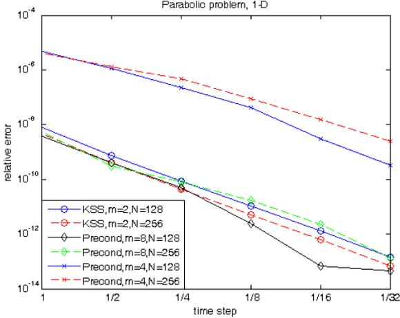
Figure 1: Estimates of relative error at  $t = 0.1$  in solutions of (11) computed using preconditioned exponential integrator [30] with 4 and 8 Lanczos iterations, a 4th-order method based on an exponential integrator [15], and a 2-node block KSS method. All methods compute solutions on an  $N$ -point grid, with time step  $\Delta t$ , for various values of  $N$  and  $\Delta t$ .
