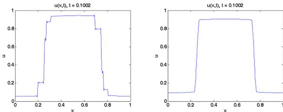
Figure 5: Sharpening of a smooth function, using  $c = 1$ ,  $\varepsilon = 0.1$ ,  $\Delta t = 0.0003$ . Left plot: backward Euler with MINRES for time-stepping. Right plot: KSS method.
